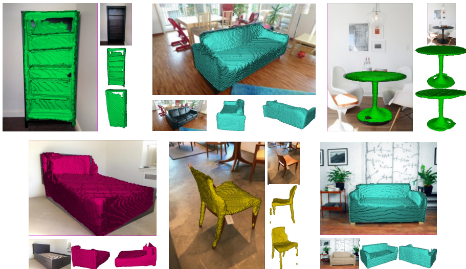
Fig. 5: Qualitative results on Pix3D. For each example, the large image shows our reconstruction overlaid on the RGB input. The smaller images show the RGB input, and our reconstruction viewed from two additional viewpoints.
