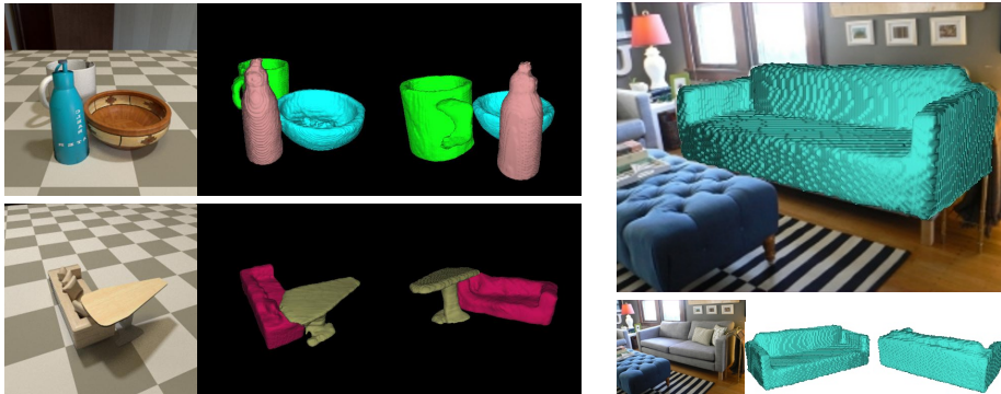
Fig. 1: 3D reconstructions from a single RGB image, produced by our model. Left: Coherent reconstruction of multiple objects in a synthetic scene (shown from a view matching the input image, and another view). We reconstruct all objects in their correct spatial arrangement in a common coordinate frame, enforce space exclusion, and hallucinate occluded parts. Right: Reconstructing an object in a real-world scene. The top image shows the reconstruction overlaid on the RGB input. The bottom row shows the input next to two other views of the reconstruction.
